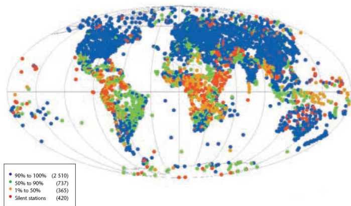
Figure 15 The global network of the World Weather Watch (WWW) stations colour coded to indicate silence (red dot) or reporting rates in 2004. Source: WMO (2005)
